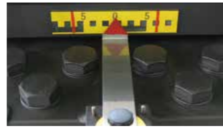
Bearing position indicator
