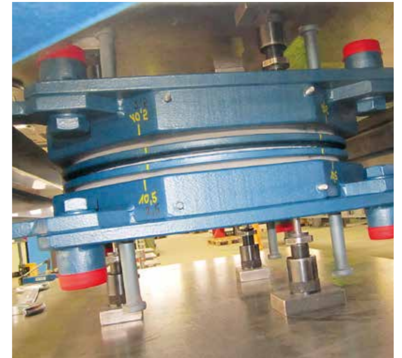
Final quality inspection of the free sliding pot bearing
