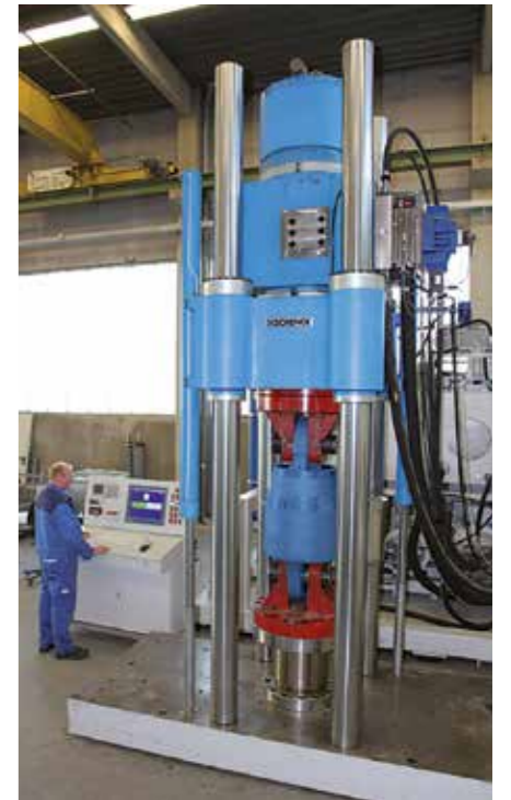
Dynamic testing of a viscous fluid damper in the SCHREIBER testing laboratory
