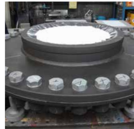
Cap fixture with sliding material SMS®
