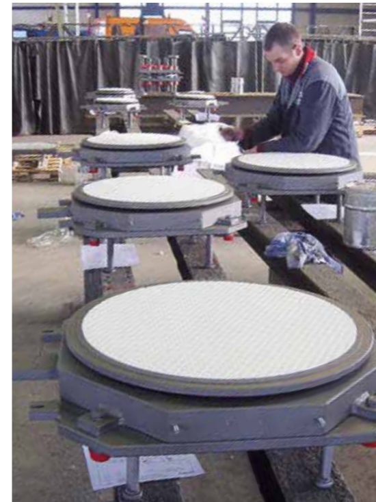
Assembly of free sliding pot bearings
