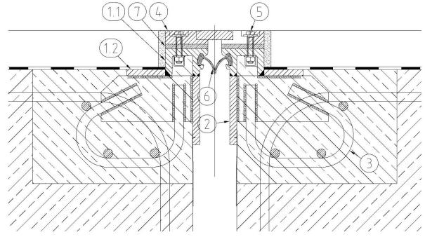
Figure 4: Exemplary cross section of the nosing expansion joint
