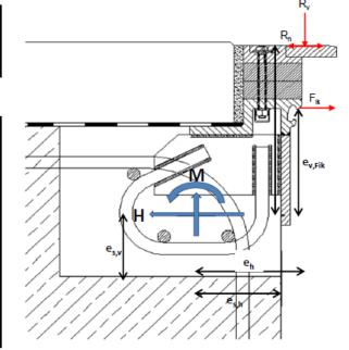
Note: The two lines indicating the forces transferred to the anchorage are taking into account the horizontal loads acting in both directions.
