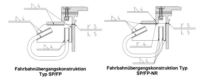
Figure 5: Dimension and type of welds according to EN ISO 2553
